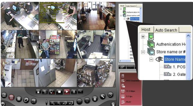
**11** When you click the **+** sign, a list of cameras will drop down. You will be able to drag and drop any of these cameras in any of the camera boxes on the left or double click on the host name.
